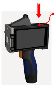
Insert cartridge to printer by an angle of 15 degree. Press vertical when insert right position, then hear "click", that means the cartridge already is fixed well.
